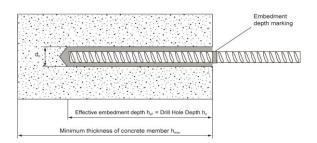
Table A2: Installation details for rebar
